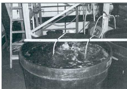
Artificial seawater being mixed in preparation for laboratory-scale testing of ballast water treatment systems carried out for the MARTOB project.
