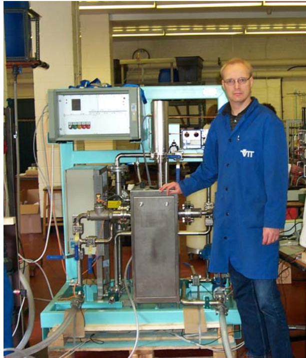
Figure 5. Laboratory scale equipment for UV and US systems
