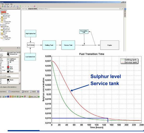
Vessels with single fuel system must pay attention to needed change over time and fuel handling procedures.
