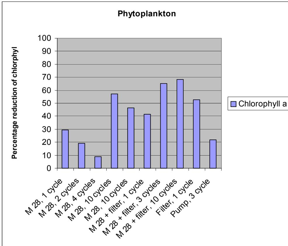
Figure 10.3. Percentage reduction of Chlorophyll a in BenRad Marine Technology water purifier.
