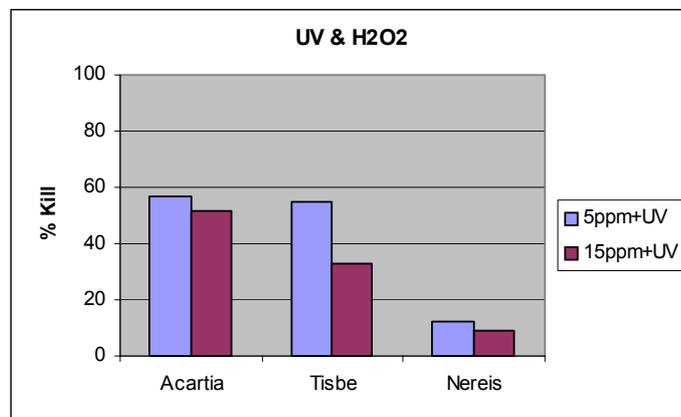
**Fig. 2** % Kill for the UV+H<sub>2</sub>O<sub>2</sub> hurdle technology, comparing 2 different concentrations.
