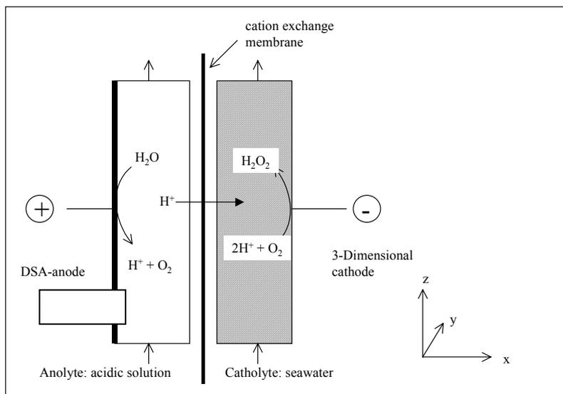
Figure 5.1. The principle of  $\text{H}_2\text{O}_2$  production by the Oxide method.
