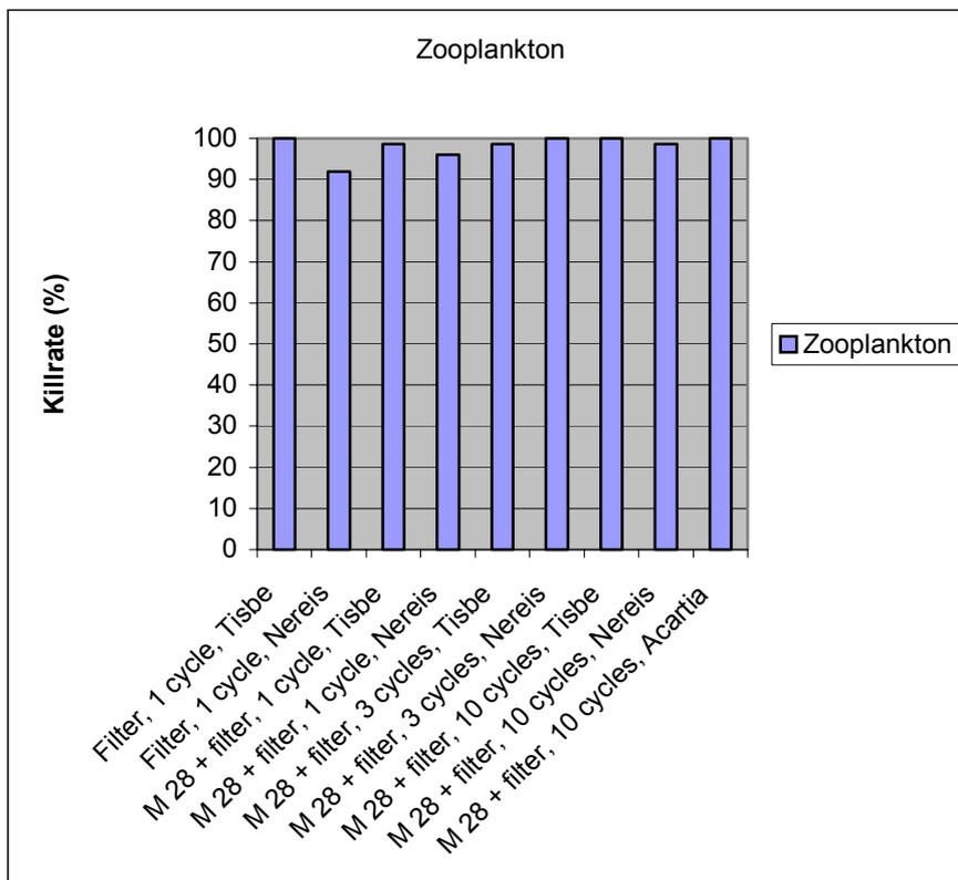
Figure 10.2. Killrate of Zooplankton in BenRad Marine Technology water purifier + 100 µ filter.
