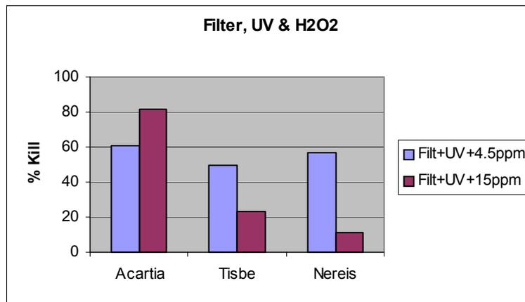
**Fig. 3.** % Kill of organisms for hurdle technology of Filter+UV+H<sub>2</sub>O<sub>2</sub>, with 2 different concentrations.
