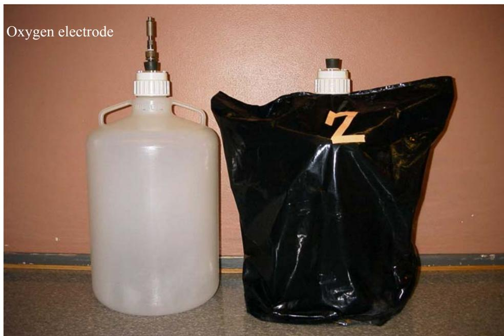
Figure 3.2. Polypropylene vessel used as "ballast tank". The vessel was closed with a silicon rubber stopper, through which an oxygen electrode was inserted into the water to measure dissolved oxygen, and covered with a black plastic bag to minimise exposure to light.
