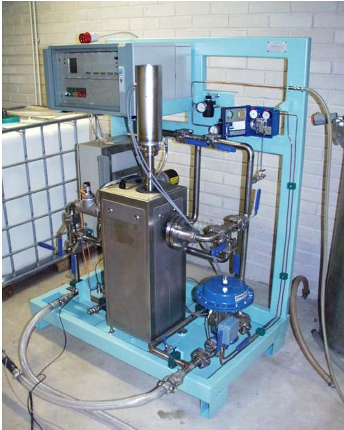
*Figure 4.2. The ultraviolet light and ultrasonic devices mounted in the same aggregate. Ultrasound transducer is mounted inside the stainless steel box.*
